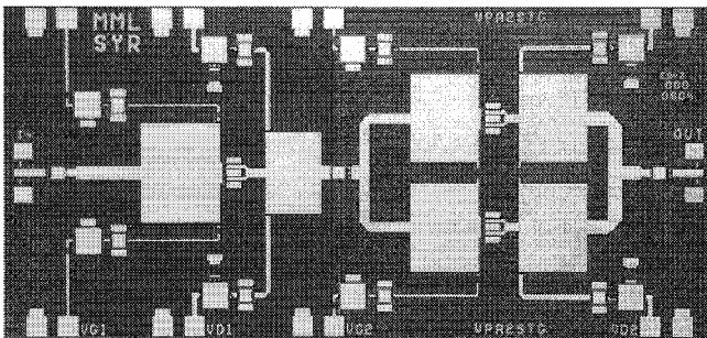
Fig. 2. Photograph of the V-band monolithic power amplifier. The chip size is  $3.39 \times 1.61 \text{ mm}^2$ .
