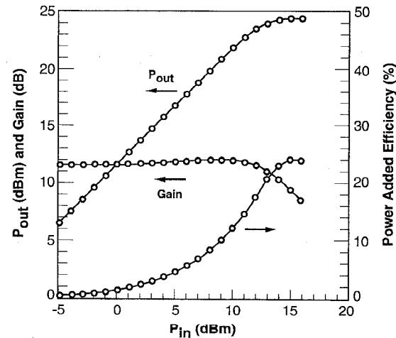
Fig. 3. Measured 60-GHz performance of the monolithic amplifier, operated with both stages at  $V_{ds}$  of 5.0 V.
