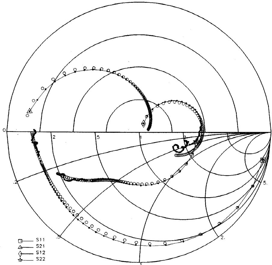
Fig. 1. Comparison of measured and modeled S-parameters of  $0.1 \mu\text{m} \times 300 \mu\text{m}$  PHEMT across 1–75 GHz frequency range. Open symbols are modeled data,  $S_{21}$  full scale is 10 and  $S_{12}$  full scale is 0.2. Bias conditions are  $V_{ds} = 4.5 \text{ V}$ ,  $I_{ds} = 42 \text{ mA}$ .
